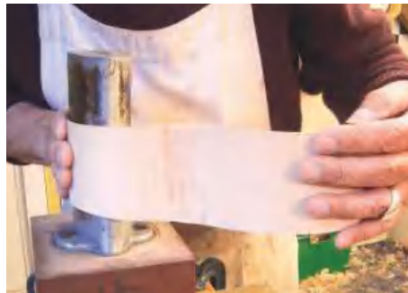
▲ Pic.11 Bending the sides on the hot iron
